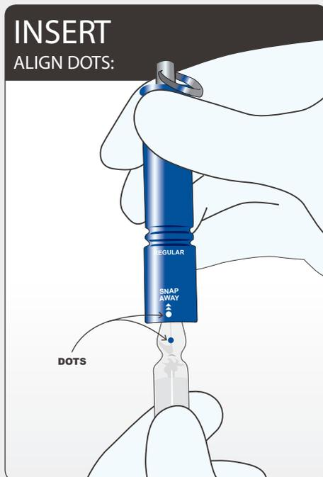
1. Align the dots if present. Gently insert all of the ampoule lid into the SnapIT. The ampoule lid becomes locked in at the neck.
